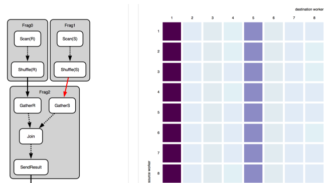
Figure 5: Worker Communication matrix chart. Each cell represents the number of exchanged tuples between a pair of workers.
